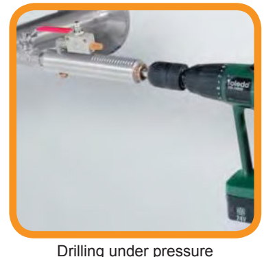
Drilling under pressure
