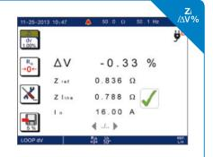
of the conductor is sufficient for the installation. The result of this  $\Delta V$  measurement is displayed in %; if the value is greater than 5 % or a programmed value, the sizes of the cables for the installation must be recalculated.
