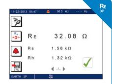
3-pole earth measurement using 2 auxiliary stakes (also known as the 62 % method) is the earth measurement of reference which yields a precise resistance value for the earth electrode.
