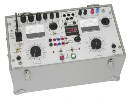
T&R Test Equipment is a market leader in the field of current injection equipment. The range includes secondary injection units with 100A output capability up to 6000A primary injection systems. All have true RMS metering, a flexible timing system, and an easy to understand user interface.
