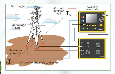
Used in conjunction with the C.A 6474 vectorial processing unit, the C.A 6472 offers the possibility of measuring a pylon's earth resistance even if it is part of a parallel earth network, by selective measurement of the pylon in question.
