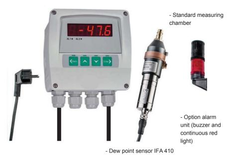
The measuring range of -80...20°Ctd makes the dew point set IDS 52 with alarm the ideal dew point monitor with analogue output 4...20 mA.
