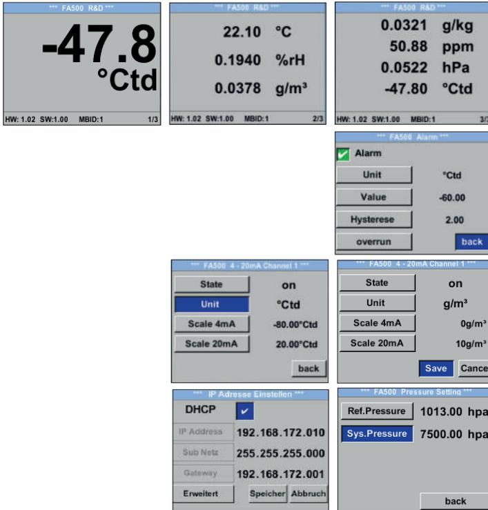
The integrated display shows the dew point in big figures as well as further humidity parameters on two more display pages. The arrow key can be used to scroll between the display pages.
