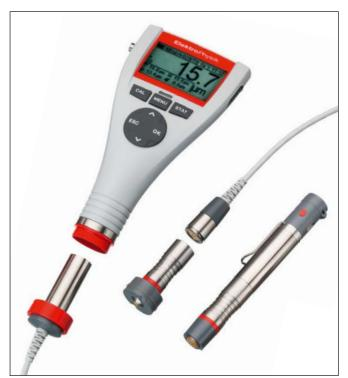
**MiniTest 745** – the top model of the series – convinces through its flexible sensor design. Its built-in sensor can be easily converted into an external sensor. Thus you can take advantage of the features of both sensor designs. Additional comfort and flexibility is provided by the wireless sensor.
