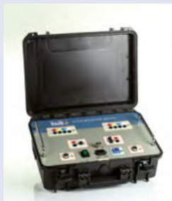
20A DC BOOSTER FOR WINDING RESISTANCE TEST
