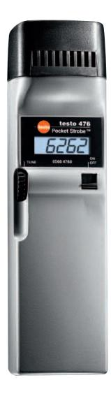
The energy-optimized switching electronics and the lightintensive xenon flash lamp provide a high light intensity (approx. 800 Lux). testo 476 has a memory function which stores the last measurement value when the instrument is switched off. For long-term inspections of measurement objects, a trigger input is available.
