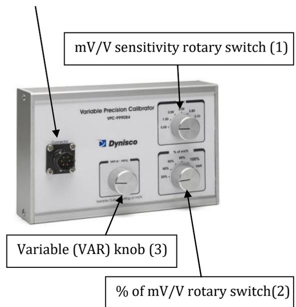
**Operation (Variable Position and "VAR" knob)** Switching the rotary switch to the position labeled "VAR" allows Infinite resolution between 0 - 100% adjustment using the rotary knob variable knob. Note that the knob is only operational when the % of mV/V rotary switch is in the "VAR" position.
