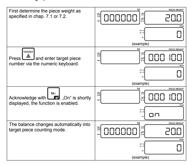
Count-in the parts, when display green and no signal sounds, the target piece number is reached.
