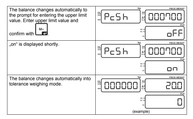
Count-in parts; when the piece number is within the tolerance range, the display background illumination changes to green.
