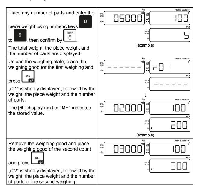
If needed, weigh-in more weighings as specified. Ensure that the balance is unloaded between the weighing procedures.
