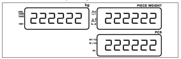
After that the balance will change automatically into the weighing mode, the zero display appears in all three display windows and the balance is now ready for operation:
