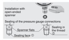
sealing face ①. With tapered threads (e.g. NPT threads), sealing is made in the threads ② using additional sealing materials, e.g. PTFE tape (EN 837-2).
