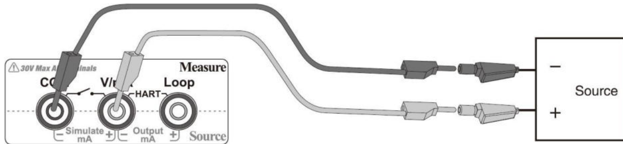
Figure 9 Current / Voltage Measurement
