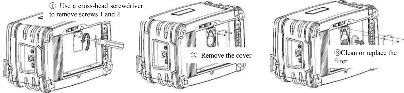
Figure 8- 1 Disassembly of the suction filter
