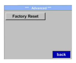
By pressing "Factory Reset" the sensor is set back to the factory settings.
