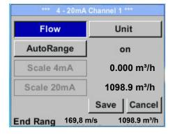
The 4-20 mA Analogue output of the Sensor IVA 570 can be individually adjusted.
