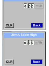
The scaling of the 4-20mA channel can be done automatically "Auto Range = on" or manual "AutoRange = off".
