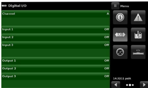
Figure 6.4.11-A - Digital I/O Application
