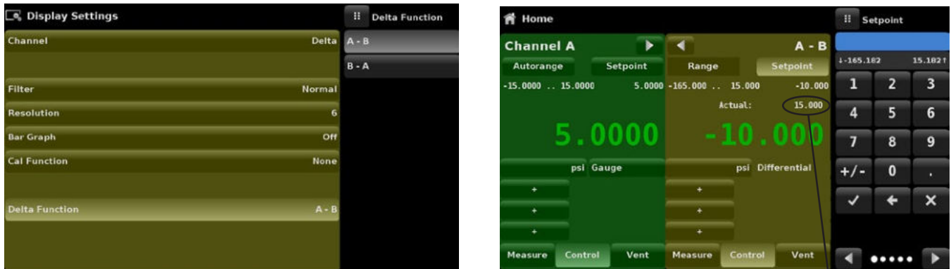
Actual pressure is shown on delta channel indicating the pressure of the physical channel.
