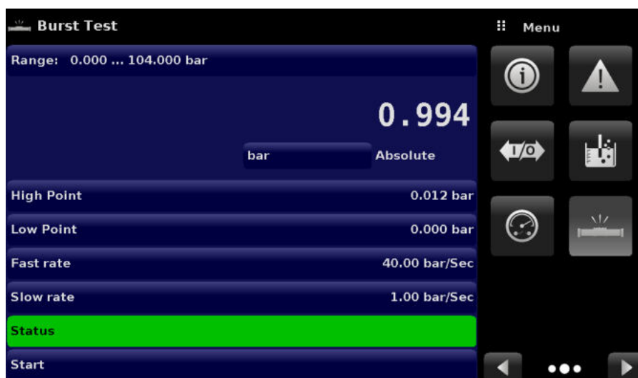
Figure 6.4.14-B Burst Test Complete (No Burst)
