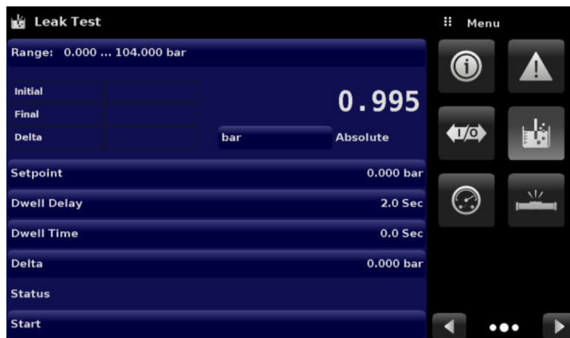
Figure 6.4.12 Leak Test App
