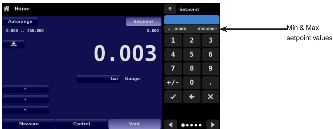
Figure 6.4.1.2.1 Numeric Keypad Setpoint Entry
