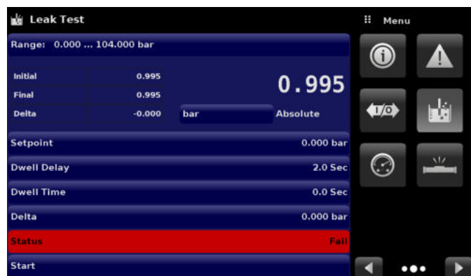
Figure 6.4.12-A Leak Test Fail (left) and Pass (right)
