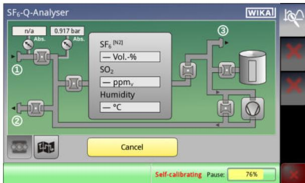
If the measuring instrument has experienced large temperature differences or if very dry gas is to be measured, the instrument must be switched on at least 1 hour before the measurement.
