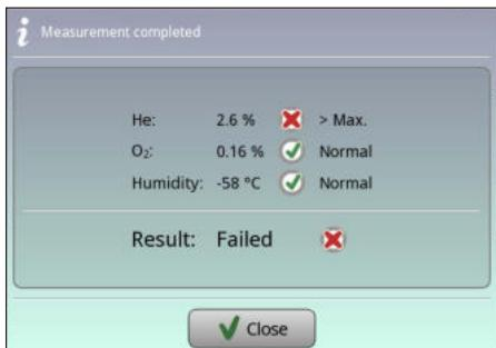
Measuring results are automatically compared with the defined limit values and an OK symbol is displayed if they pass.
