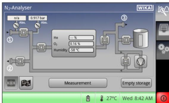
2. Select the gas compartment for pumping the measuring gas back (only available when the “pumping back” function is selected).
