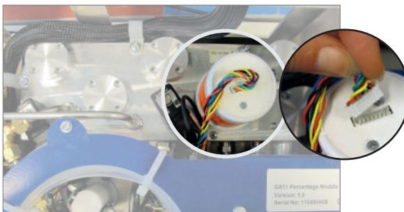
3. Screw out the sensor counterclockwise.
