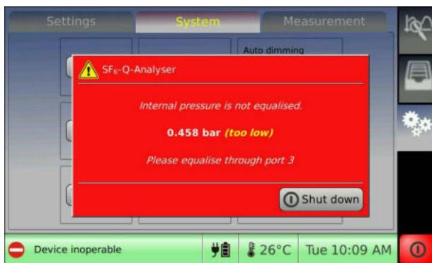
For pressure compensation, connect a gas recovery bag with the desired gas (under atmospheric pressure, max. 1,200 mbar abs. or 200 mbar rel.) to the outlet for the gas recovery bag ③.
