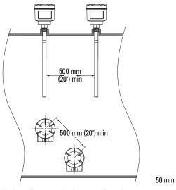
Horizontally mounted units are configured as point level switches. Mount diagonally if vertical space is restricted.
