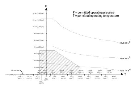
The curve denotes the minimum allowable flange class for the shaded area below.
