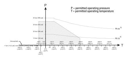
1) The curve denotes the minimum allowable flange class for the shaded area below.
