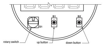
The rotary switch can be set from 0 to 5. Each position represents a menu. The position wraps from 5 to 0.
