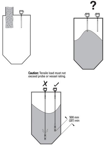
**Note:** Buildup of material or condensation in active shield area does not affect operation.
