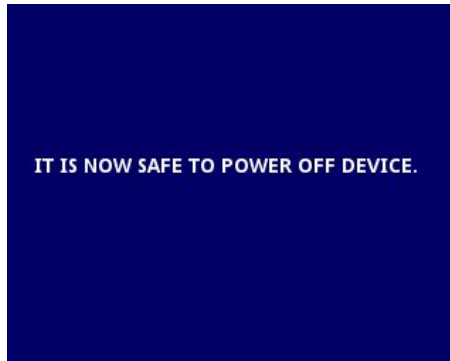
Fig. 6.1. The view of the screen after pressing the Safe shutdown button
