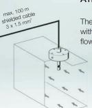
The SLF... sensor can be used in combination with an ASL... evaluation device to monitor the flow in the air (e.g. in air-conditioning systems).
