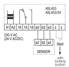
In case of malfunction, a sensor error can be ruled out by checking the resistances between the connecting wires. Sensor SLF15 must be disconnected and checked with a suitable ohmmeter between the individual connecting wires:
