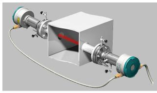
An Ex concept with type of protection "Flameproof enclosure d" is used for the SITRANS SL. The enclosure used resists an explosion caused by a potentially explosive gas mixture in the analyzer. Ignition of a potentially explosive atmosphere produced outside the enclosure is therefore reliably prevented.
