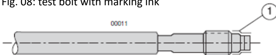
Fig. 08: test bolt with marking ink
