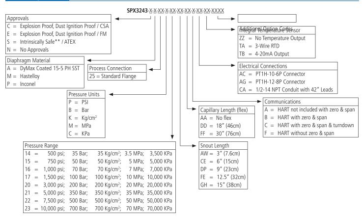
Certain configurations cannot be combined on the same unit (example: Approval "E" and Electrical Connections "AC" or "AG" are not compatible. The Ordering Guide shows only a sample of configuration options. Contact Dynisco for additional options, pricing and lead times.
