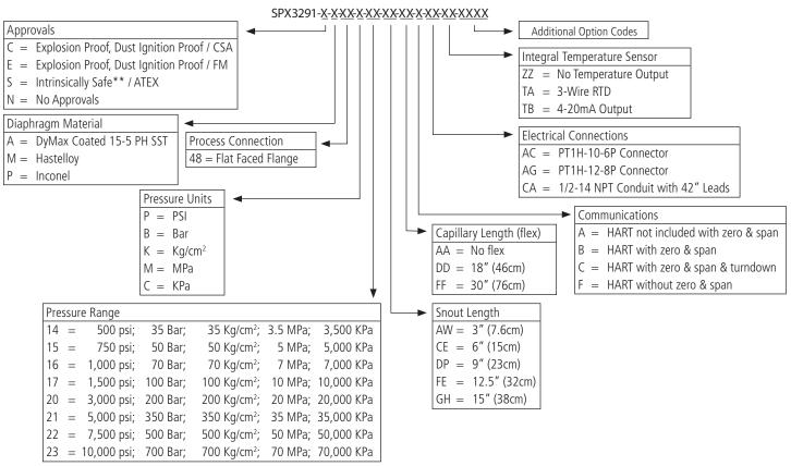
Certain configurations cannot be combined on the same unit (example: Approval "E" and Electrical Connections "AC" or "AG" are not compatible. The Ordering Guide shows only a sample of configuration options. Contact Dynisco for additional options, pricing and lead times.
